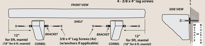
**2.** Apply mortar or construction adhesive to top of corbels and back of shelf
